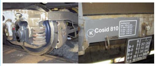
Figure 3.2.1: Picture of wagon retrofitted with k-blocks. Old wagons such as these are now as silent as modern passenger vehicles.
