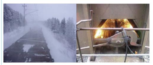
Figure 3.2.3: Testing braking performance under winter conditions and locked brake testing. Both are part of the homologation testing. Work is going on to enable the testing of these properties on test benches.
