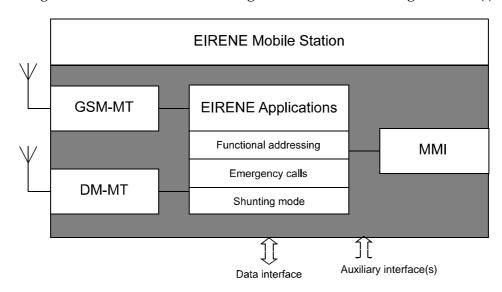
Figure 7A-1: Logical Shunting radio architecture and interfaces
