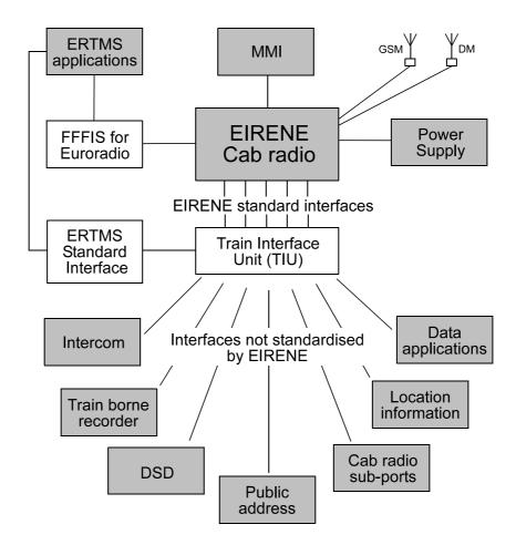
Figure 5-3: Interfaces to the Cab radio
