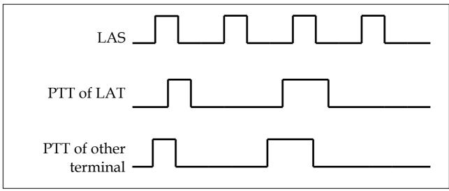
Figure 14-9: LAS in point-to-point mode, including more then one PTT.
