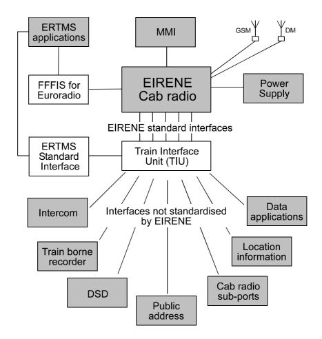
Figure 5-3: Interfaces to the Cab radio
