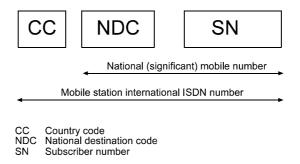
Figure 9-3: Number structure of MSISDN number
