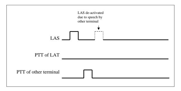
Figure 14-5: LAS in group mode, Terminating Mode 1.
