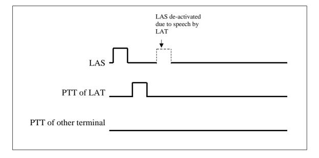
Figure 14-6: LAS in group mode, Terminating Mode 2.
