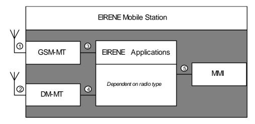
Figure 4-1: Logical mobile radio architecture and interfaces
