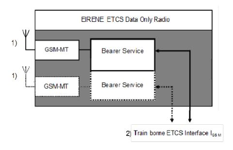
Figure 16-1: Logical ETCS data only radio architecture and interfaces
