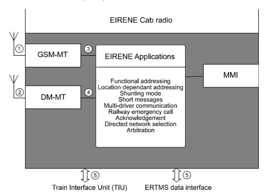
Figure 5-1: Logical Cab radio architecture and interfaces
