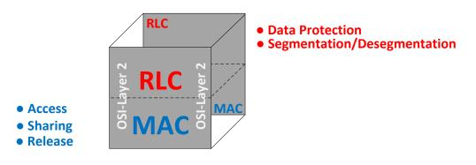
Figure 2-4 GPRS Protocol Stack - RLC/MAC transport functions
