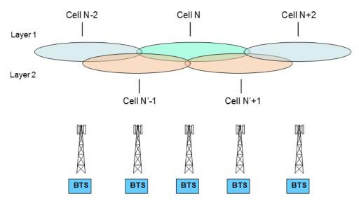
Figure 2-12 Dual Radio Layer Coverage – with layer offset
