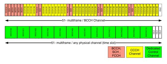
Figure 2-15 Logical Channel sequence non-combined channel setup - Downlink
