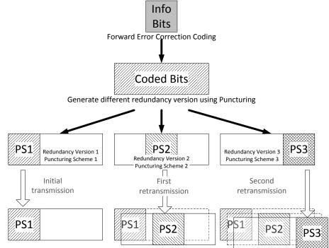
Figure 2-8 Incremental redundancy principle
