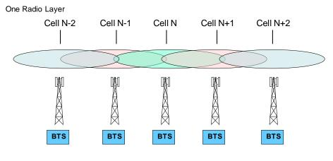
Figure 2-10 Single radio layer architecture – extended adjacent cell overlapping
