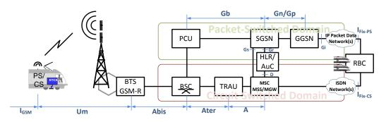
Figure 2-1 GSM-R logical network architecture including CS- and PS-Domain
