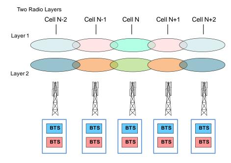
Figure 2-11 Dual Radio Layer architecture – no layer offset
