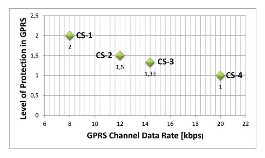
Figure 2-6 Link between FEC and the resulting Channel Data rate in GPRS
