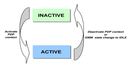
Figure 8-1 PS-mode - Functional PDP state model
