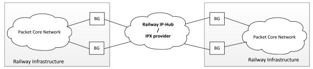
Figure 8-2 Point of Interconnection between IP-hub and the local Packet Core network
