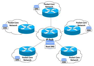
Figure 6-1 PS-mode Roaming - IP-hub
