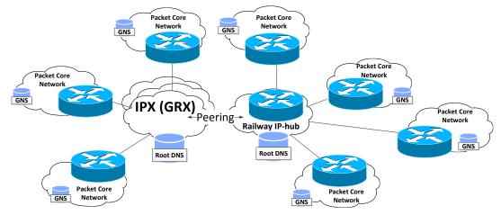
Figure 6-2 IP-hub - IPX peering schematic
