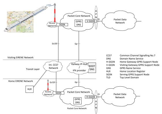
Figure 8-1 Network Architecture Interworking PS-mode roaming
