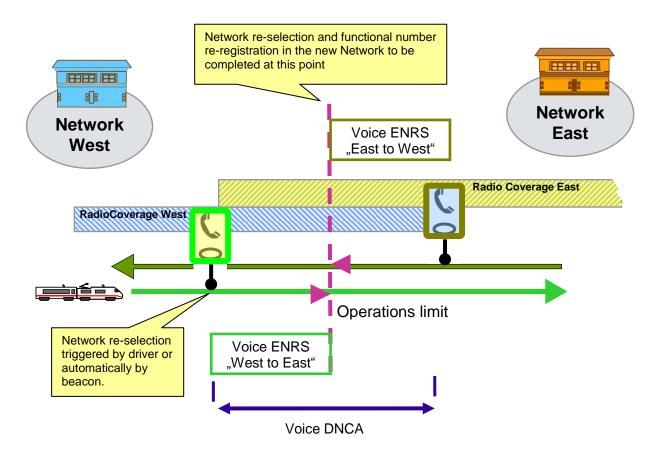
Figure 1: Dual Network Coverage Zone at EIRENE network borders without ETCS)
