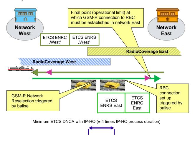
Figure 4: Minimum DNCA including ETCS and use of IP-HO
