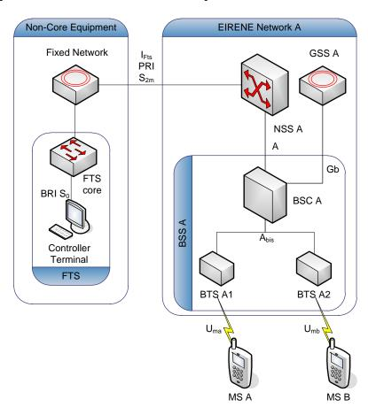
Figure 1a: Reference testing architecture single network
