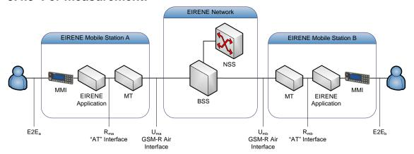
Figure 8: Measurement architecture
