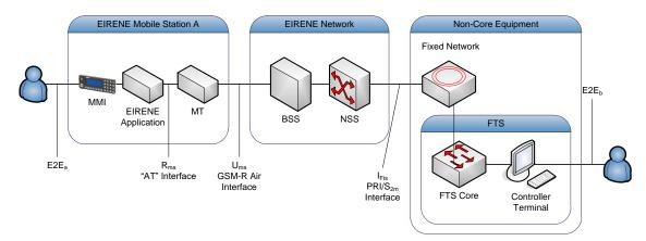
Figure 13: Measurement architecture
