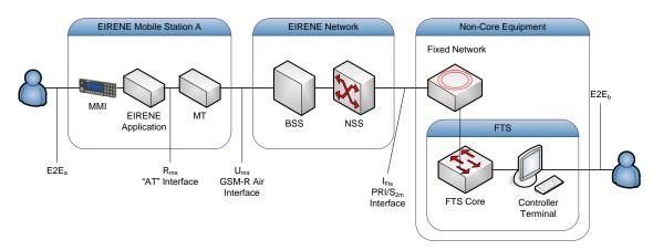
Figure 11: Measurement architecture
