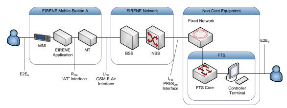
Figure 6: Measurement architecture
