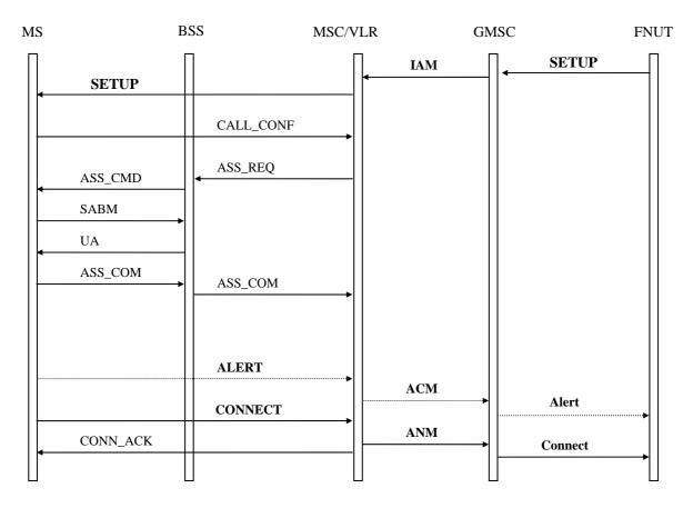
Figure 3: Signalling flow for a mobile terminating call
