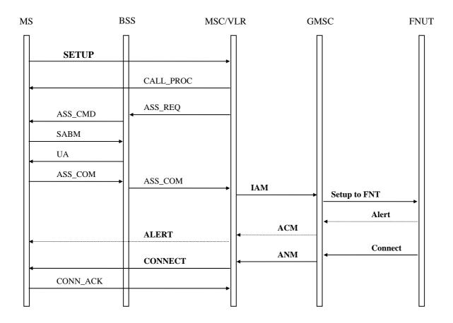
Figure 2: Signalling flow for a mobile originating call
