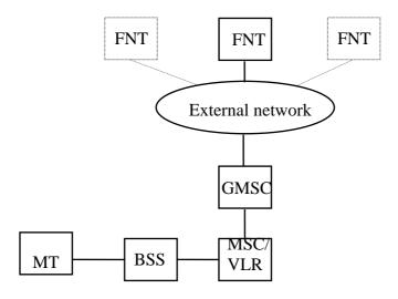
NOTE: The functional architecture is only indicative. The MSC and GMSC may also be collocated and FNT may also be connected directly to the MSC using a PABX.
