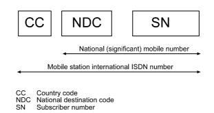
*Figure 9-3: Number structure of MSISDN number*
