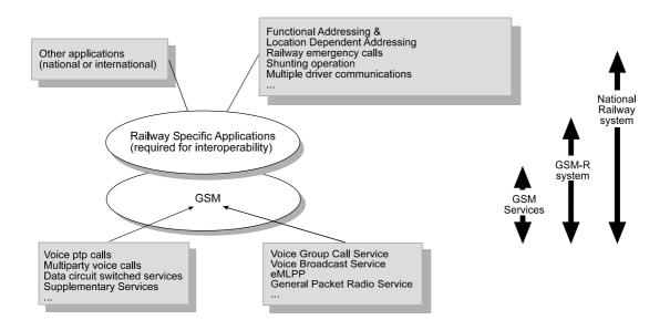
Figure 1-2: Scope of the GSM-R system with reference to functionality provided by GSM
