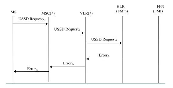
Fig. 3: Information flow for mobile initiated failed USSD Request on HLR
