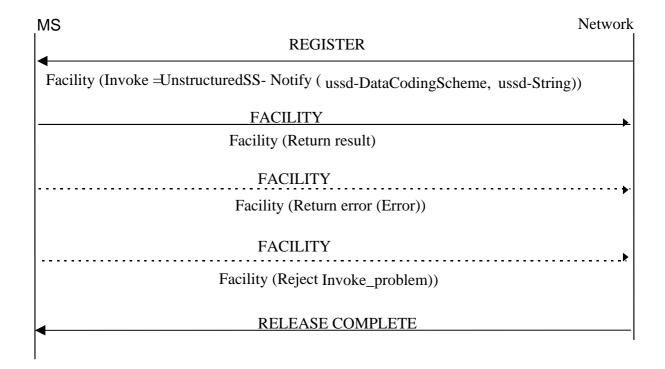
Fig. 5: Single network initiated USSD operation
