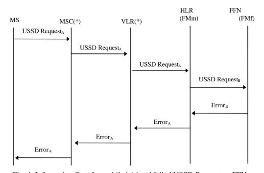
Fig. 4: Information flow for mobile initiated failed USSD Request on FFN.
