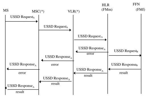
Fig. 2: Information flow for mobile initiated USSD Request containing FM related operations
