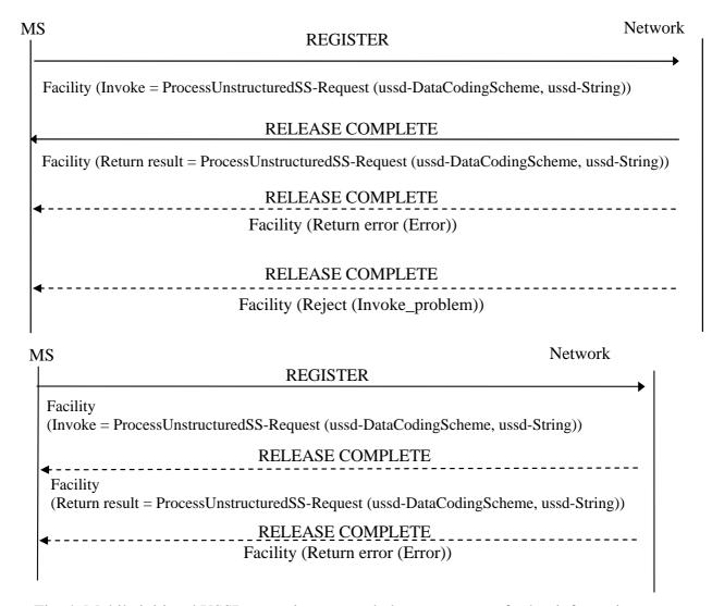
Fig. 4: Mobile initiated USSD operation, network does not request further information
