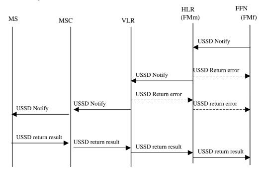
Fig. 2: Information flow for network initiated USSD Request containing deregistered functional number
