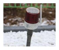
"A smart measurement system that consists of a rod-shaped displacement sensor, IoT client, and gateway to measure the slope displacement in the vicinity of the slip surface. It is an intelligent sensor-based slope failure early warning system that transmits a real-time warning to the users if the rate of displacement exceeds the standard value set by the algorithm."<sup>21</sup>
