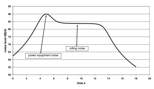
Figure 3 : noise level time history for diesel hauled train (80km/h, d = 25m)
