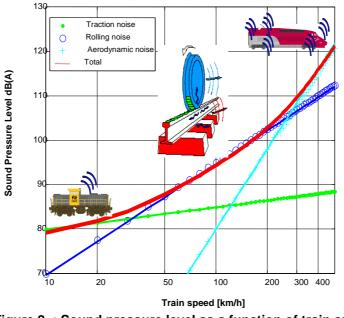
Figure 2. : Sound pressure level as a function of train speed
