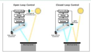
Figure 2: Categories of automatic daylight harvesting lighting controls. Source: IntelliBlinds.
