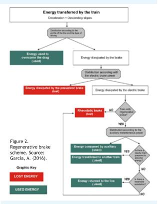
In the case of AC electrification or in DC lines with reversible substations, the energy returned to the catenary, first of all is used by other trains (if any) and if there are not trains, it is fed back into the public grid (see figure 3).
