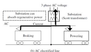
Figure 3. Regenerated energy flow in each electrified line. Source: Keiichiro Kondo (2010).
