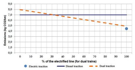
Figure 4. CO<sub>2</sub> emissions according to the electrified length in passenger transport. Source: Gonzalez Franco, I et al. (2010).
