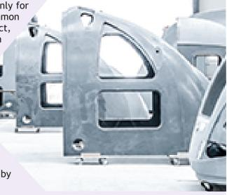
Figure 1: Composite train cab. Source: Alcan Airex Composites.
