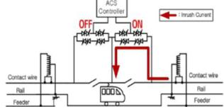
Figure 5. Electric railway system with ACS system and SFCL.. Source: Hee-Sang Shin (2011).
