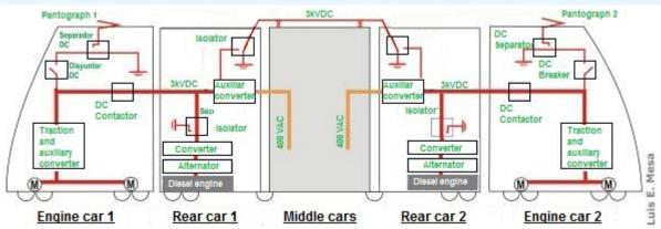
Figure 3. Dual passenger train supplied by diesel. Source: Gonzalez Franco, I et al. (2010).
