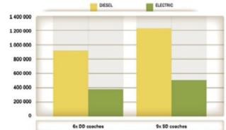
Figure 5. Energy cost per train and year in diesel in electric traction. Source: Railway Hand Book (2015).
