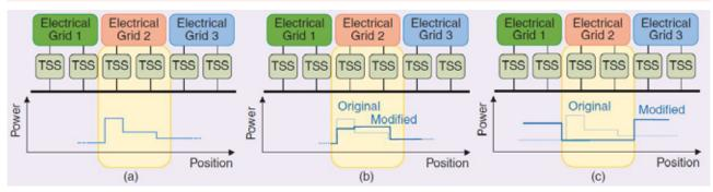
Figure 3. The different driving changes executed to manage the power demand in an RPS: (a) base case, (b) power peak reduction, and (c) energy transfer. Source: Pilo, E. et al. (2014).
