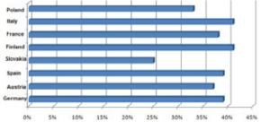
on 5% 10% 15% 20% 25% 30% 35% 40% 45% Figure 3. Thermal power plant efficiency. Source: García, A. (2016).
