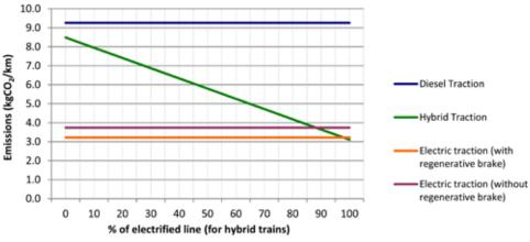
Figure 5. CO<sub>2</sub> emissions according to the electrified length in freight transport. Source: Gonzalez Franco, I et al. (2010).
