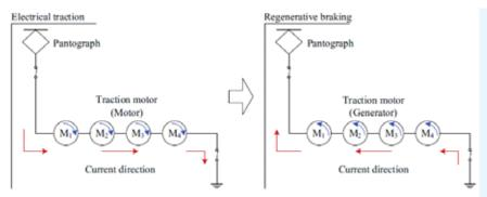
Figure 1. Principle of regenerative braking. Source: Xin Yang, et al (2015).
