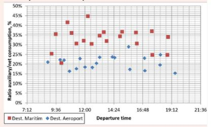
Figure 2: Ratio between auxiliary and net energy consumption in two lines of the Valencia Metro Network. Source: Martínez et al. (2015).
