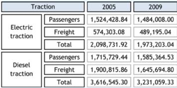
Table 1. Energy consumption according to the traction. Source: Own elaboration by UIC data. (2016).
