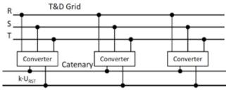
Figure 3. Power-supply system using converter . Source: Pilo, E. (2014).
