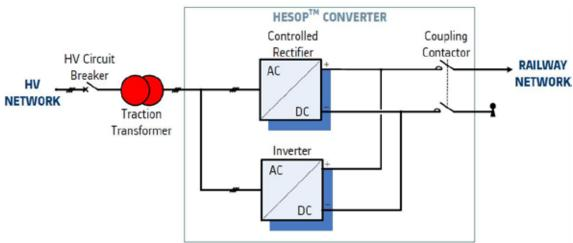
Figure 8. Architecture of the prototype power converter. Source: Cornic, D. (2010).
