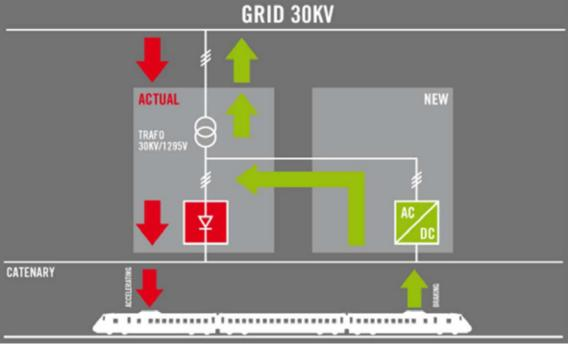
Figure 7. Reversible substation scheme. Source: Romo, A (2015).
