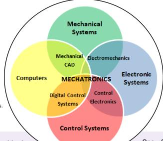
Figure 1: Relationship between mechatronics and other systems. Source: Own elaboration.
