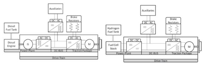
Figure 2. Diesel-electric drive system. Source: Hoffrichter, A (2013).
