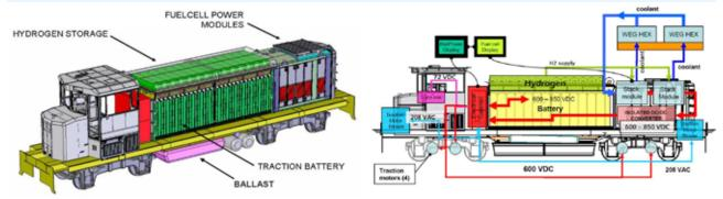
Figure 4. Hydrogen fuel cell CAD model Source: Miller, A. R. (2007).
