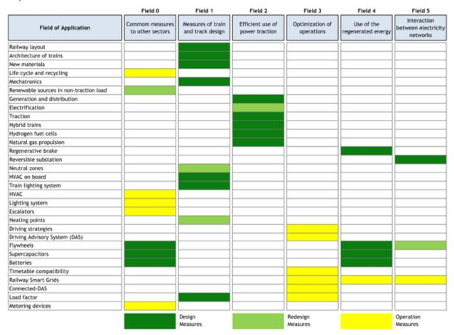
Table 1. Measures for energy consumption reduction and emissions in the railway classified by field of application. Source: Independently produced (2016).
