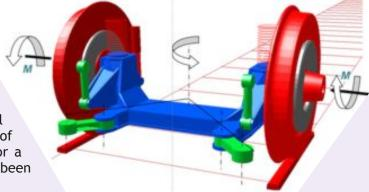
Figure 2: Unit with carrier and independently torque-controlled wheels for the mechatronic running gear. Source: Robotics and Mechatronics Center.
