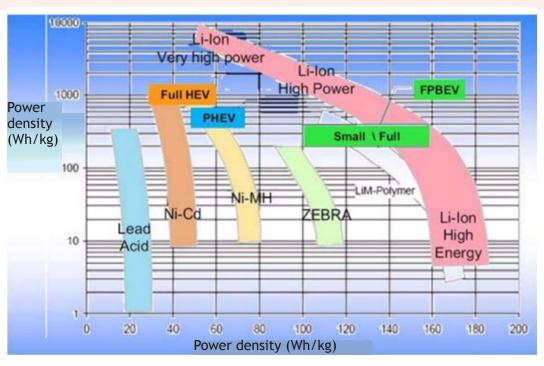
Figure 4: Relative power/energy density for different types of battery. Source: Estévez, P. et al. (2008).
