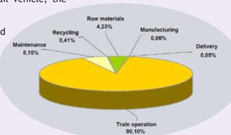
Figure 3: Energy consumption of a rail vehicle for the overall life cycle and 30 years of operation. Source: Siemens Transportation Systems (2006).
