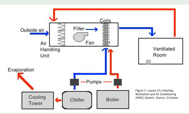
One of the elements that require most energy is the pumps, which are used to circulate hot, chilled and condensed water. Newer pumps are far more efficient and may save about 20% of energy (Asian Development Bank, 2015) compared to traditional pumps. Another energy-consuming element is the cooling tower used for heat rejection, which usually equips its own fans and pumps. Newer, hybrid cooling towers are more efficient than traditional ones.
