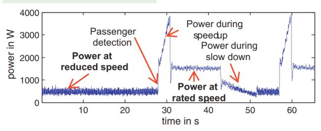
Figure 2: Power consumed by an escalator with two speed modes. Source: Carrillo et al. (2013).
