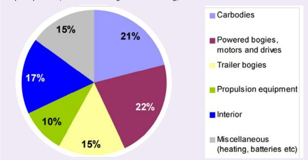
Figure 3: Typical breakdown of components in electric multiple unit trains by weight. Source: UIC EVENT (2003).
