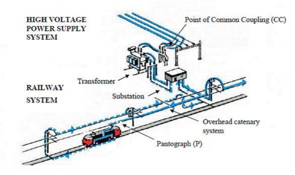
Fig. 4: Railway System and position of the Substation
