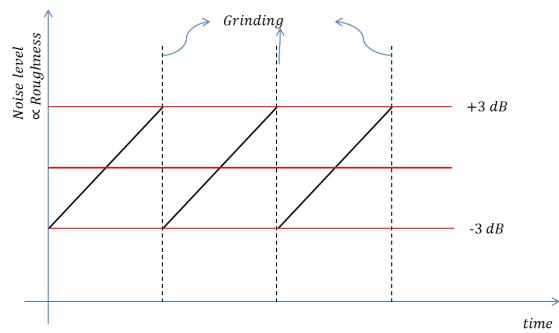
Figure 10: Evolution in time of the rail roughness by applying acoustic grinding procedure. In this model linear grow of roughness and proportionality between noise and roughness are assumed. The BüG procedure in Germany is based on this model and grinding is done when the noise level is exceed by 3 dB.
