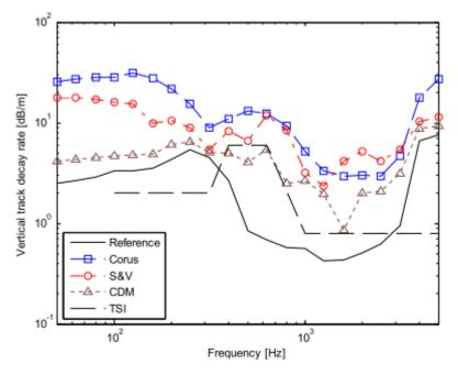
Figure 3: Example of TDR spectrum of track with dampers (figure from Qcity report<sup>1</sup>)
