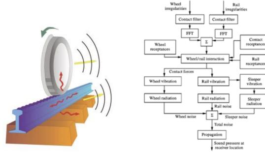
Figure 1 (left): Noise creation mechanism. Figure 2: Diagram of the noise creation in TWINS model.
