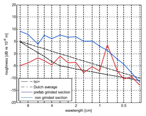
Figure 4: Example of roughness spectrum (Figure from M+P Report<sup>2</sup>).
