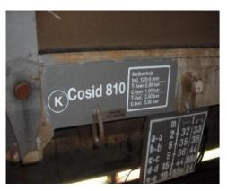
Figure 3.2. Picture of wagon retrofitted with k-blocks. Old wagons such as these are now as silent as modern passenger vehicles.
