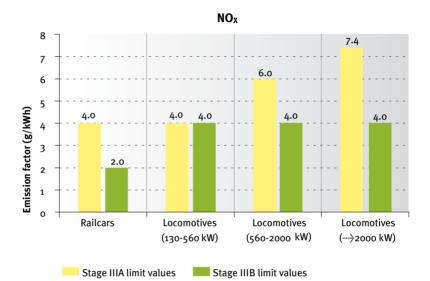
Stage IIIA and Stage IIIB emission limits
